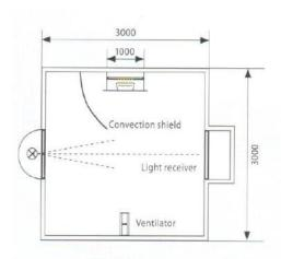
For low smoke zero halogen cables, cable Standards in general have the requirement of light transmittance that the ability to light reached 60%, the value set basis is to ensure that people can find their way in the smoke. Qualified low smoke zero halogen material and cable design can meet this requirement, however PVC base material of the cable is difficult to achieve this index, so if the projects require for cable light transmittance are not recommended to use the PVC cable.
